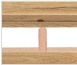
Solid dowel joint
