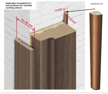
COVERING TRIMS (101) AND QUADRANT (1C1) CAN BE APPLIED TO A BLOCK DOOR FRAME FOR DOOR LEAVES IN WIDTHS "60"—"90". IN CASE OF DOOR LEAVES IN WIDTH "100" YOU HAVE TO ORDER DOUBLE COVERING TRIM OR DOUBLE QUADRANT (LC2).
