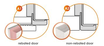
The edge of a **rebated door** leaf is finished with a rebate (visible in the picture A1) that overlaps a door frame when the door is closed. Door leaves made this way do not fit flush with a door frame.
